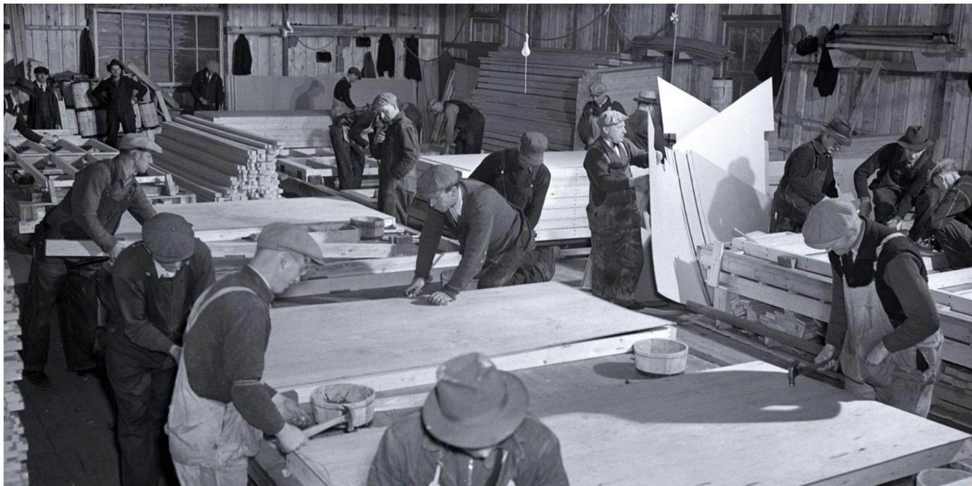
North Halifax production of pre-fab floor panels. Public Archives of Nova Scotia, 1941
