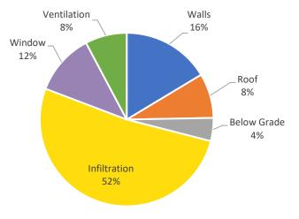
Figure 6.2 - Enclosure Heat Loss Breakdown
