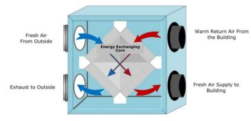
Figure 8.1 Example of Energy Recovery Ventilator
