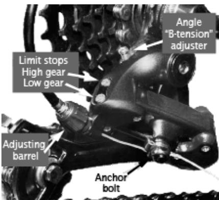
difference on a bike with indexed shifting, because the cable will not let the derailleur overshift past the smallest sprocket. If it is too tight, you it will be difficult or
