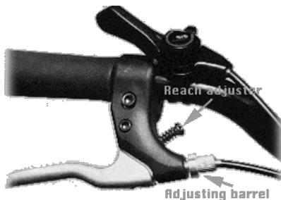
in closer to the handlebar for easier operation by a rider with short fingers.
